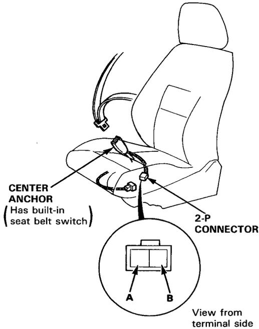
2. There should be continuity between the A and B terminals when the seat belt is not buckled. There should be no continuity when the seat belt is buckled.
