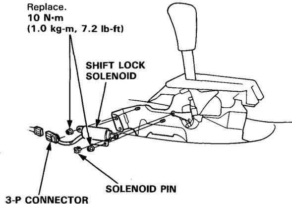
3. Install the shift lock solenoid in the reverse order of removal and adjust its position.
