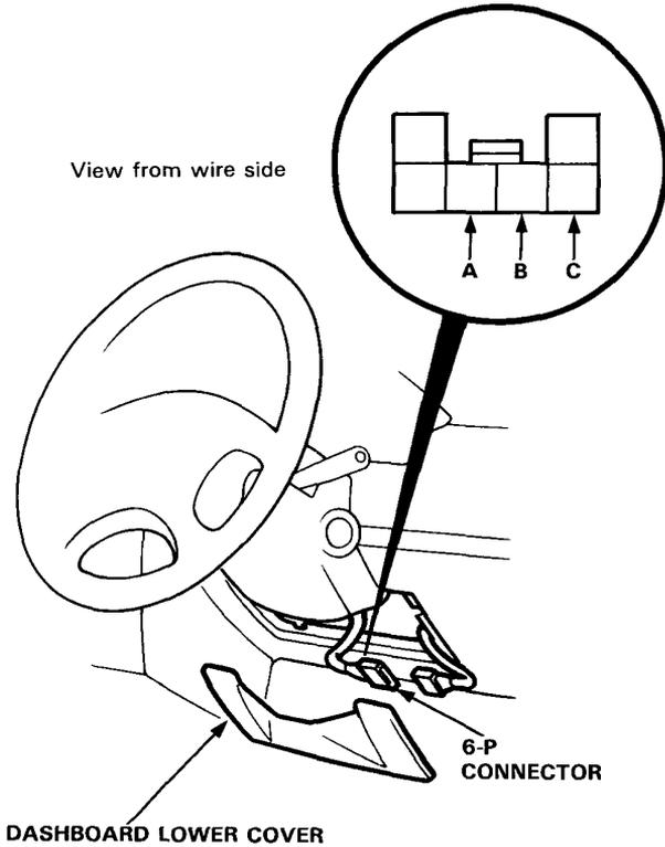
3. Check for continuity between the terminals in each switch position according to the table.
